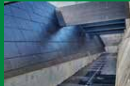
Wear liners to suit material being handled
