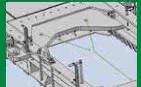
Pulling points to allow manual opening
