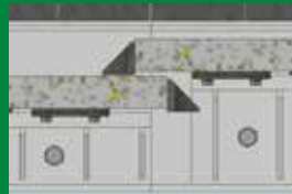
Plates overlap to minimise material leakage
